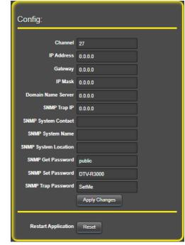
f) Use the IpSetup software you downloaded earlier to search for devices on the network. Once you find your device, open a browser and type in the IP address IpSetup found. Username: admin Passwork: Dtvx. From there you can go to the "config" page to set a static IP address assigned supplied by the network admin. 1. Type in the IP information where the zero's are. 2. Click Apply Changes, and you will lose connection and need to type the new IP address in your browser.
